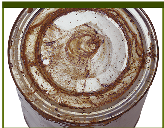
Rust that cannot be wiped off
