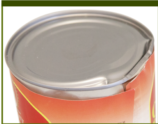
Severe dent in seam
